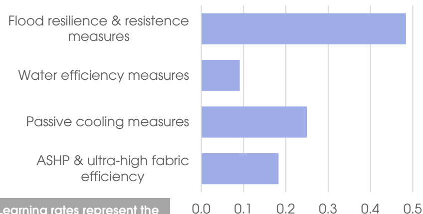
Ratio of cost of green measures in new build and retrofit for equivalent outcome United Kingdom, 2020
